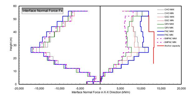
Figure 6.4-35. Tower-abutment interface normal forces
