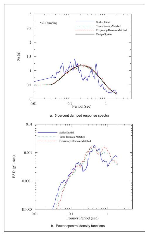
Figure C-15. Comparisons of response spectra and power spectral density functions for the scaled Gazli recording (component 090E), 1976 Gazli earthquake, and the spectrum-compatible acceleration time-histories
