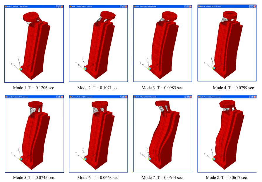
Figure 6.4-14 Vibration mode shapes
