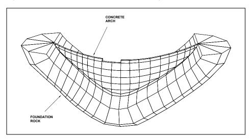
Figure 2-5. Perspective view of dam-foundation finite element model
