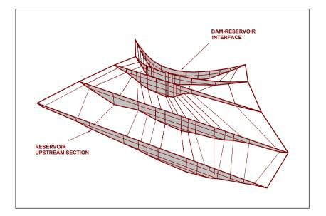
Figure 6.2-6. Finite element model of incompressible reservoir water
