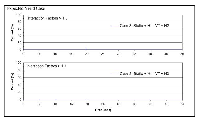
Figure 4-33 Peak percentage of H-piles whose combined interaction factor values exceed 1.0 and 1.1; expected yield case; lower miter gate monolith for MDE
