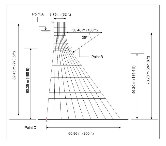
Figure 6.1-3. Section geometry and finite element model
