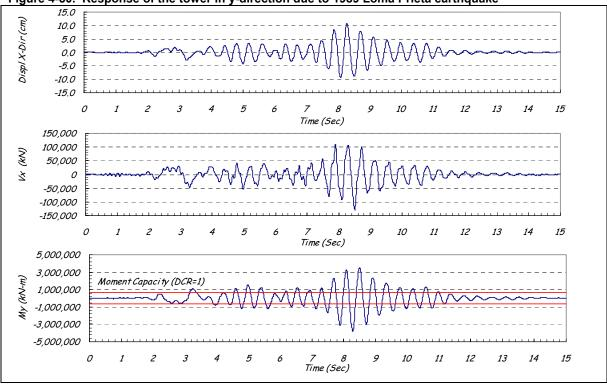
Figure 4-50. Response of the tower in y-direction due to 1989 Loma Prieta earthquake
