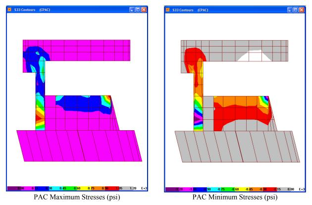
Figure 6.4-23. Vertical stresses in right face of high-level intake for PAC
