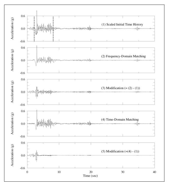
Figure C-1. Comparison of time-histories for Petrolia recording (component 000E), 1992 Cape Mendocino earthquake (Sheet 1 of 3)
