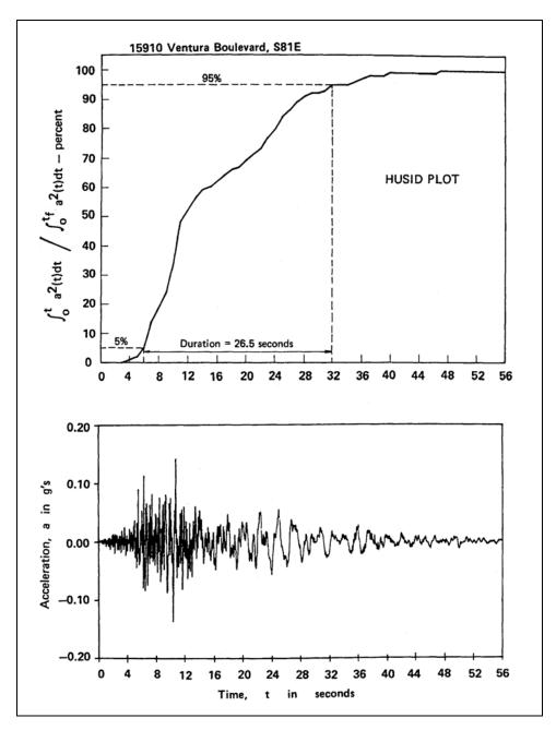
Figure 5-3. Typical Husid plot and duration as defined by Trifunic and Brady (1975) and Dobry, Idriss, and Ng (1978) (from Idriss 1979, courtesy of American Society of Civil Engineers)
