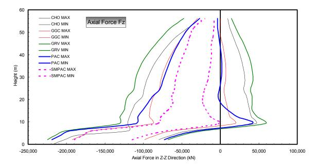
Figure 6.4-31. F<sub>z</sub> (vertical) axial force diagram (+ = tension, - = compression)
