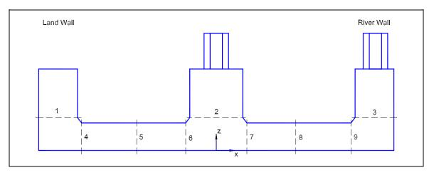
Figure 4-34. Critical lock sections for assessment of forces and moments
