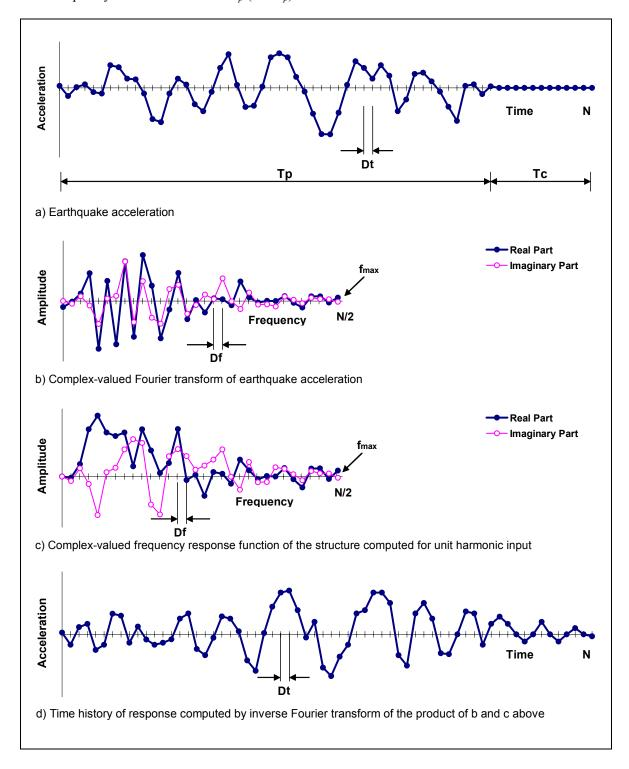
Figure 3-1. Phases of dynamic response computation in frequency domain and relationships between response parameters
