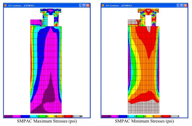
Figure 6.4-20. Normal stress contours at tower-abutment interface for SMPAC
