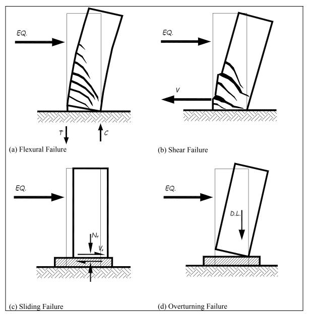
Figure 4-37. Probable modes of failure for free-standing towers where EQ. = lateral earthquake load, T = tensile base reaction force, C = compressive base reaction force, V = base shear,  $N_f$  = normal force at the base,  $V_f$  = shear friction , and D.L. = dead load
