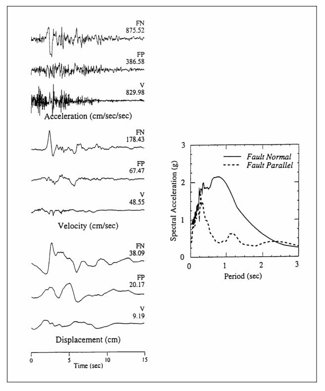
Figure 5-4. Time-histories and horizontal response spectra (5 percent damping) for the strike-normal and strikeparallel components of ground motion for the Rinaldi recording obtained 4.5 miles (7.5 km) from the fault rupture during the 1994 Northridge, California, earthquake (Somerville 1997)
