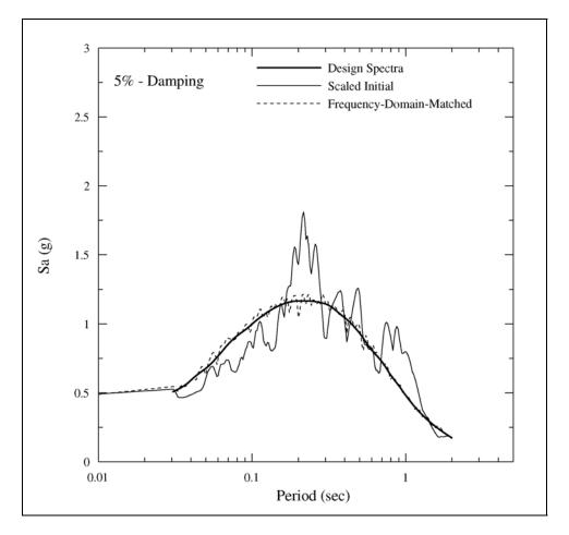
Figure 5-9. Comparisons of response spectra from the scaled 1971 San Fernando earthquake at Griffith Partk (270E) and the frequency-domain matched acceleration time-history
