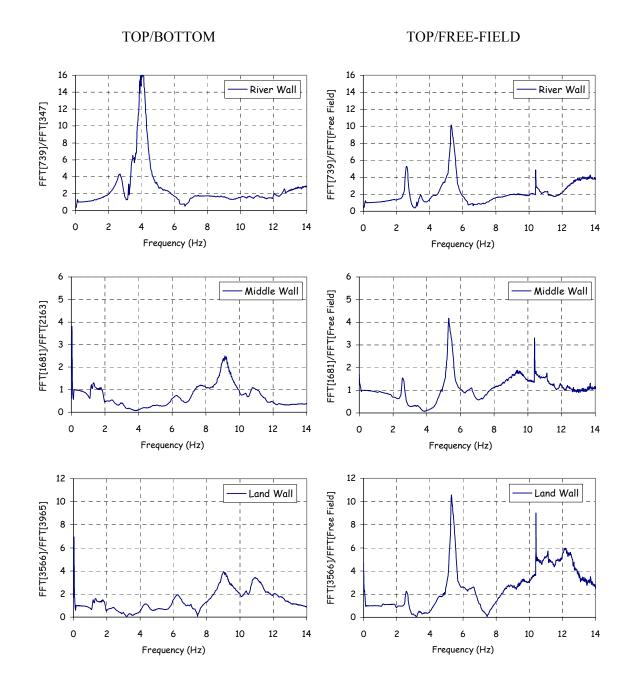
Figure 6.3-14. Transfer functions between top and bottom of lock walls, and top of lock walls and free field ground surface
