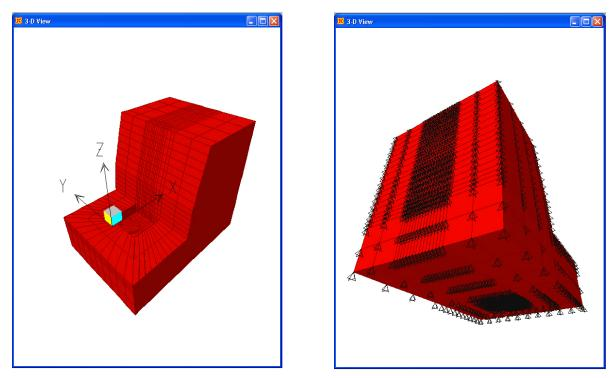
Figure 6.4-12. 3-D views of foundation-abutment finite-element model
