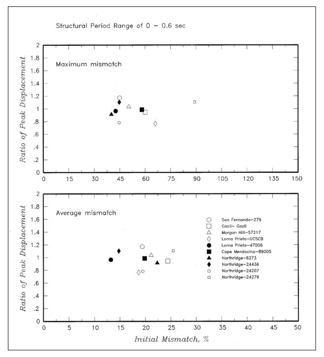
Figure D-46. Relationship between initial mismatch and peak displacment ratio of spectrally matched and scaled time-histories
