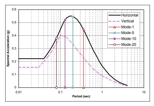
Figure 6.2-1. Horizontal and vertical smooth response spectra for MCE, M6-1/2 at distance of 18 km on the Salinas Fault (5 percent damping)
