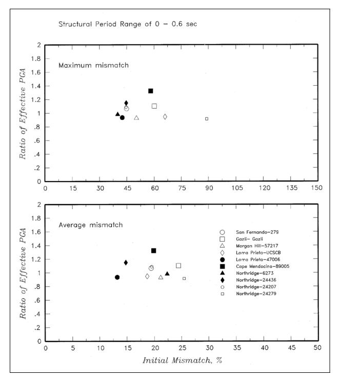
Figure D-43. Relationship between initial mismatch and effective peak acceleration ratio of spectrally matched and scaled time-histories
