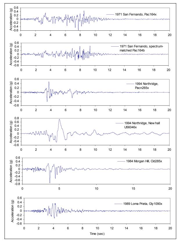
Figure 4-10. Scaled acceleration time-histories for near-source,  $M_w$ ~6-1/2 earthquake
