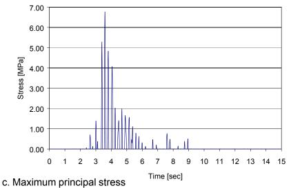
Figure 6.1-7. Relative displacement and absolute acceleration time-histories at the crest, and maximum principal stress history at point B (Loma Prieta ground motion)
