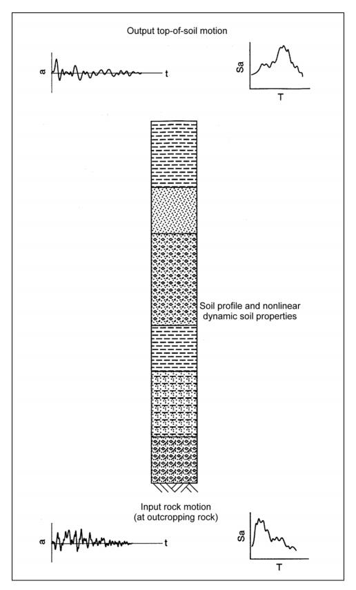
Figure 5-10. Schematic of one-dimensional site response analysis
