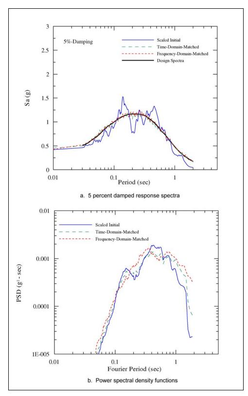
Figure C-20. Comparisons of response spectra and power spectral density functions for the scaled UCSC BRAN recording (component 090E), 1989 Loma Prieta earthquake, and the spectrum-compatible acceleration time-histories
