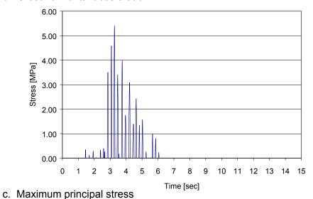
Figure 6.1-9. Relative displacement and absolute acceleration time-histories at the crest and maximum principal stress history at point B (Whittier Narrows ground motion)
