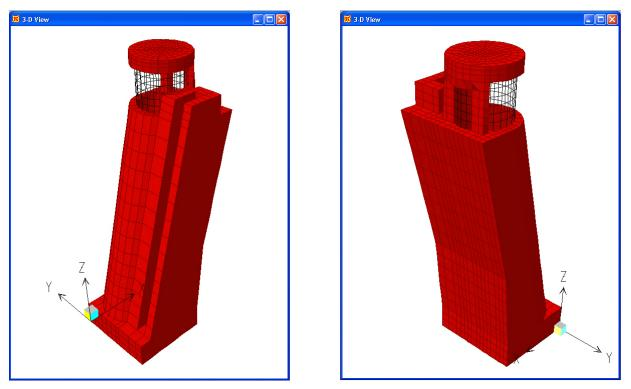
Figure 6.4-13. 3-D views of tower finite-element model
