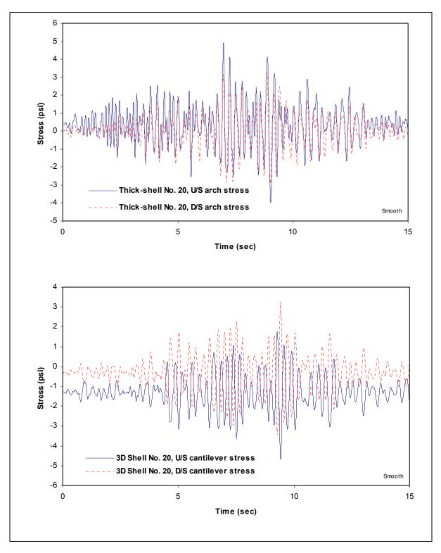
Figure 6.2-23. Time-histories of maximum arch and cantilever stresses and corresponding stresses on opposite face of the dam due to spectrum-matched record plus static loads
