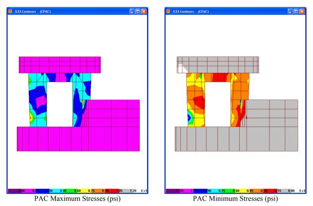
Figure 6.4-25. Vertical stresses in front face (upstream) of high-level intake for PAC
