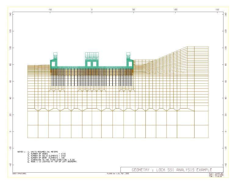
Figure 6.3-3. Finite-element mesh representation of the soil-pile-lock system
