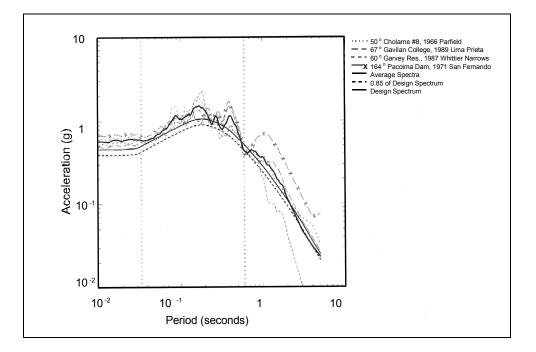
Figure 6.4-4. Target and scaled spectra, y-direction
