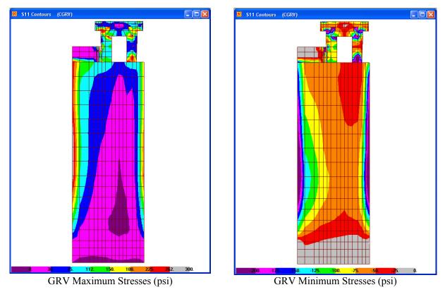
Figure 6.4-18. Normal stress contours at tower-abutment interface for GRV
