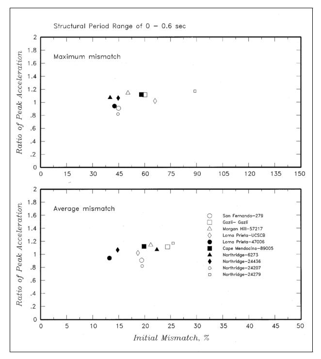
Figure D-42. Relationship between initial mismatch and peak acceleration ratio of spectrally matched and scaled time-histories
