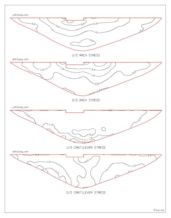
Figure 6.2-12. Envelopes of maximum stresses due to Sturno record plus static loads
