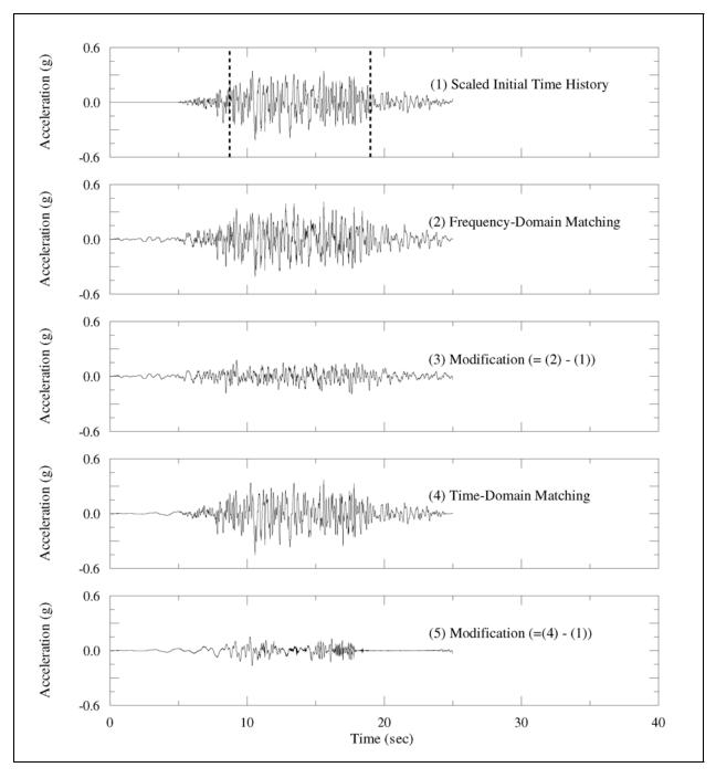
Figure C-10. Comparison of time-histories for UCSC BRAN recording (component 090E), 1989 Loma Prieta earthquake (Sheet 1 of 3)
