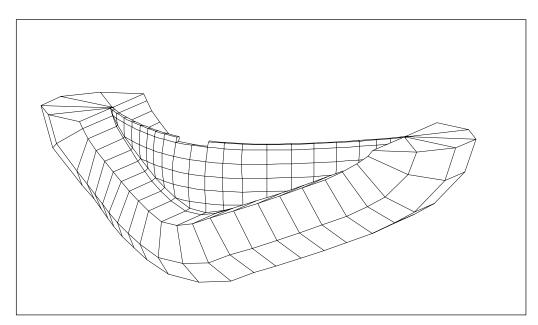
Figure 6.2-5. Finite element representation of Portugues Arch Dam and foundation rock
