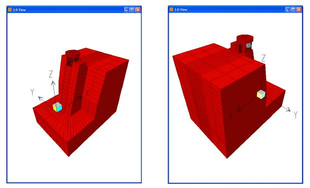
Figure 6.4-11. 3-D views of tower-foundation-abutment finite-element model
