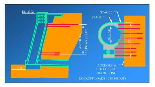
Figure 6.4-2 Seven Oaks Intake Tower Anchorage System (Courtesy of Ray Dewey, Portland Distrcit)
