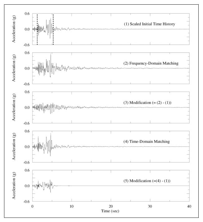
Figure C-7. Comparison of time-histories for Coyote Lake Dam recording (component 195E), 1984 Morgan Hill earthquake (Sheet 1 of 3)
