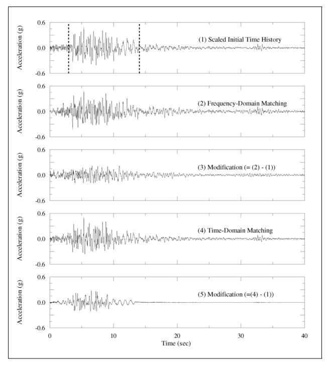
Figure C-3. Comparison of time-histories for Griffith Park recording (component 270E), 1971 San Fernando earthquake (Sheet 1 of 3)
