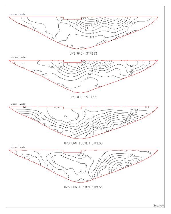
Figure 6.2-14. Concurrent stresses due to Bagnoli record plus static loads at the time of maximum arch stress
