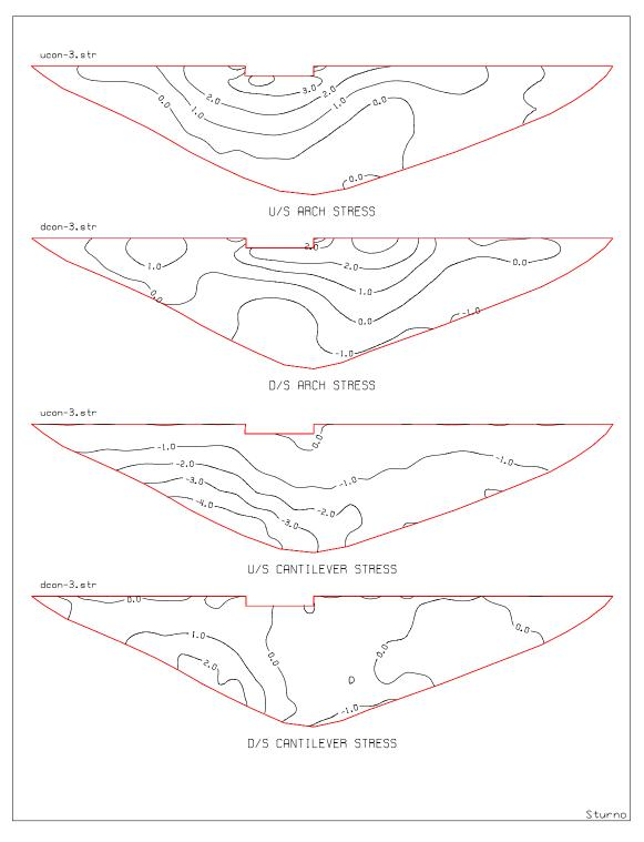
Figure 6.2-17 Concurrent stresses due to Sturno record plus static loads at the time of maximum arch stress
