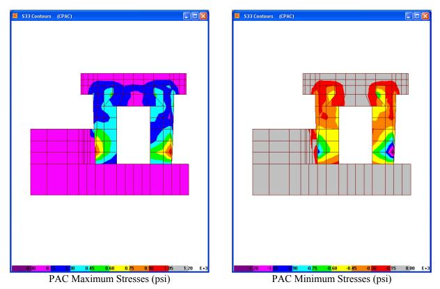
Figure 6.4-21. Vertical stresses in back face (downstream) of high-level intake for PAC
