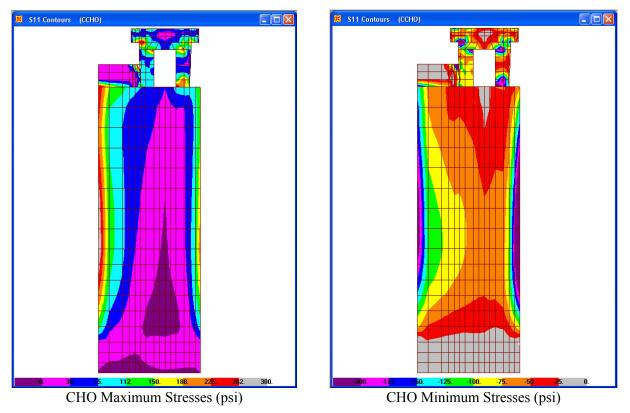
Figure 6.4-16. Normal stress contours at tower-abutment interface for CHO
