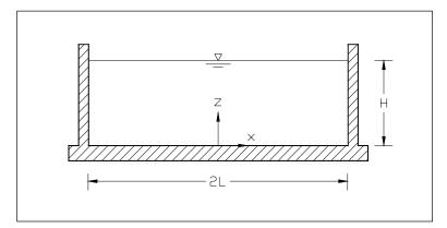
Figure 2-17. Lock chamber dimensions and coordinate system
