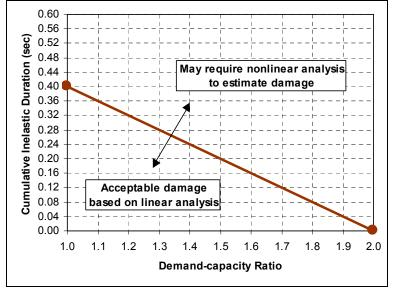
Figure 4-22. Performance curve for linear elastic analysis of arch dams
