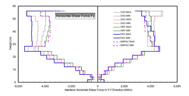
Figure 6.4-36. Tower-abutment interface horizontal shear forces
