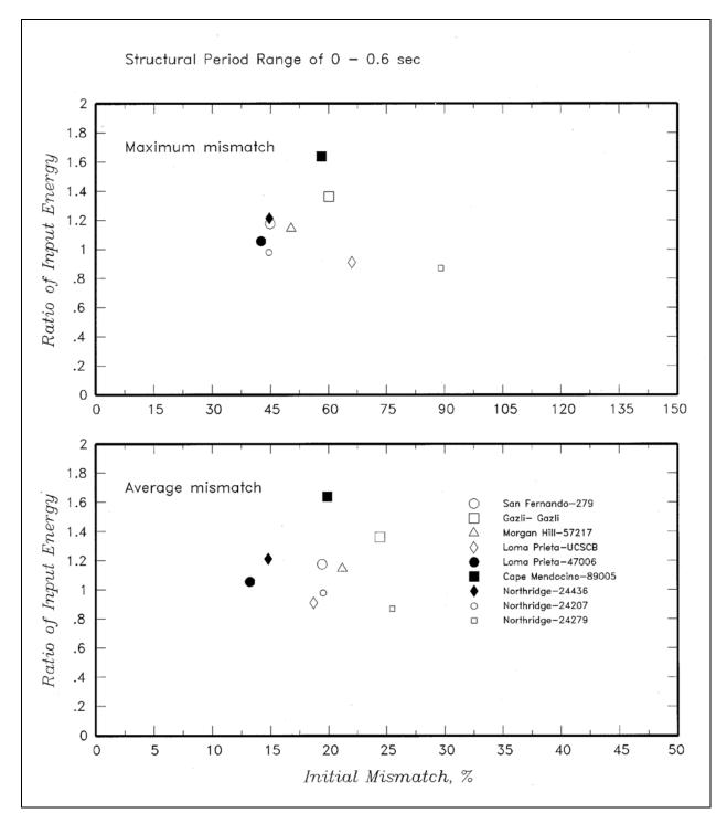
Figure D-51. Relationship between initial mismatch and input energy ratio of spectrally matched and scaled time-histories
