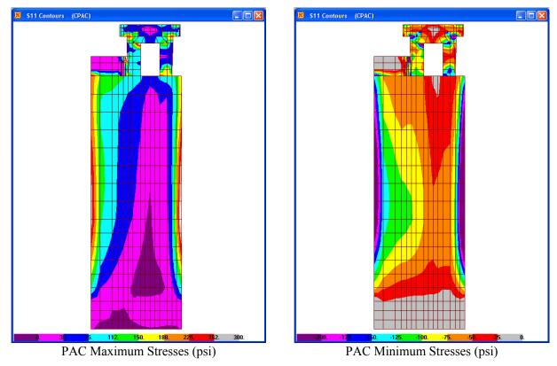
Figure 6.4-19. Normal stress contours at tower-abutment interface for PAC
