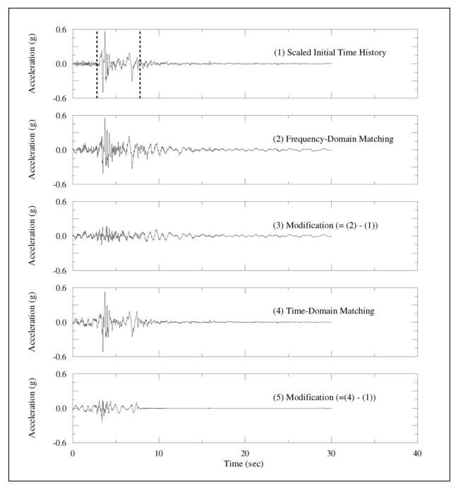
Figure C-6. Comparison of time-histories for Pacoima Dam recording (component 265E), 1994 Northridge earthquake (Sheet 1 of 3)
