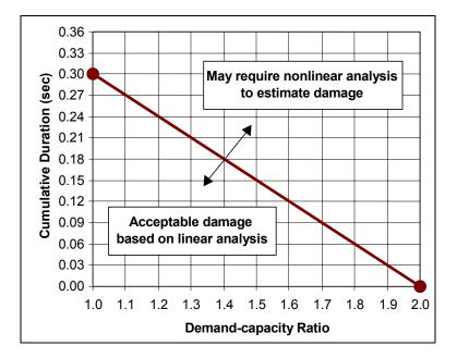
Figure 4-6. Performance curve for concrete gravity dams
