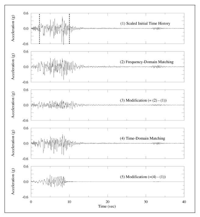
Figure C-9. Comparison of time-histories for Pacoima Dam recording (component 254E), 1971 San Fernando earthquake (Sheet 1 of 3)
