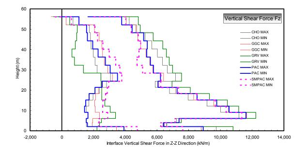
Figure 6.4-37. Tower-abutment interface vertical shear forces
