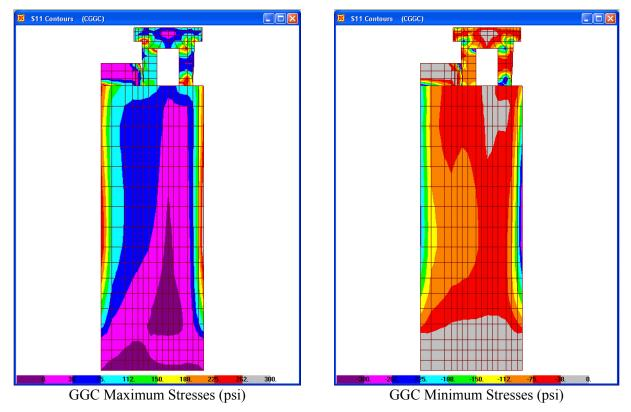
Figure 6.4-17. Normal stress contours at tower-abutment interface for GGC
