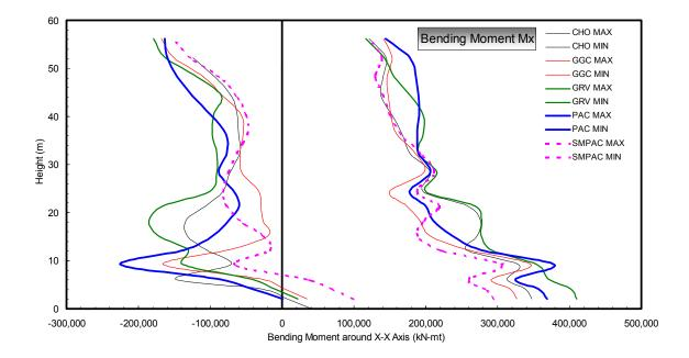
Figure 6.4-32. M<sub>x</sub> bending moment diagram
