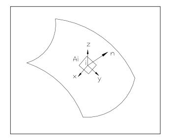
Figure 2-16. Normal and Cartesian directions of curvilinear surface
