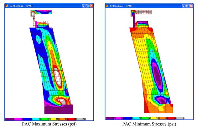
Figure 6.4-24. Vertical stresses in right face of tower for PAC
