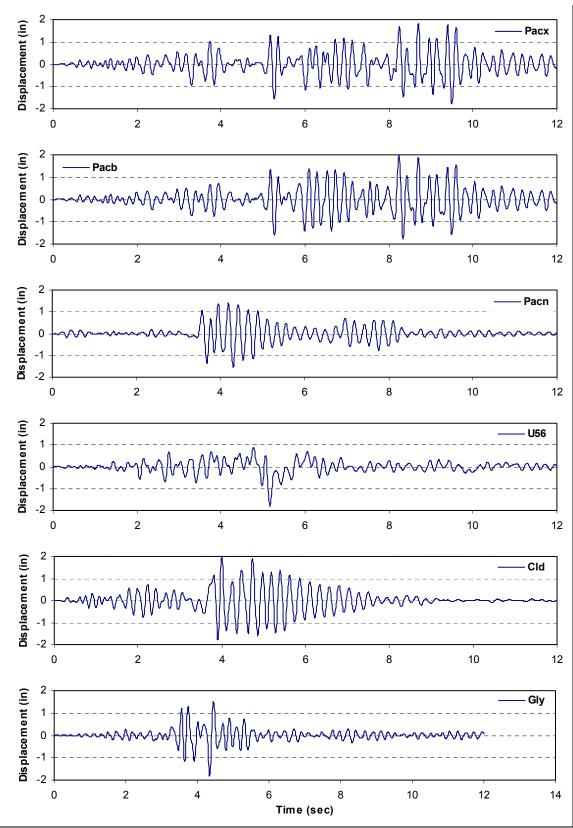
Figure 4-12. Time-histories of midcrest radial displacements for Dam-1
