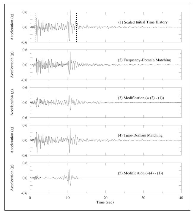
Figure C-4. Comparison of time-histories for Halls Valley recording (component 240E), 1984 Morgan Hill earthquake (Sheet 1 of 3)
