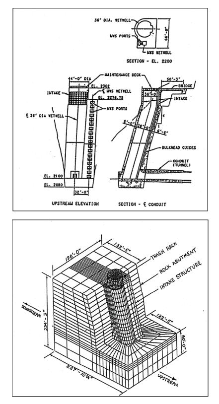
Figure 2-10. Seven Oaks Dam intake structure and associated finite element idealization (U.S. Army Engineer District, Los Angeles, 1992)
