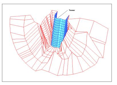
Figure 2-24. Boundary element added-mass model of Seven Oaks intake tower
