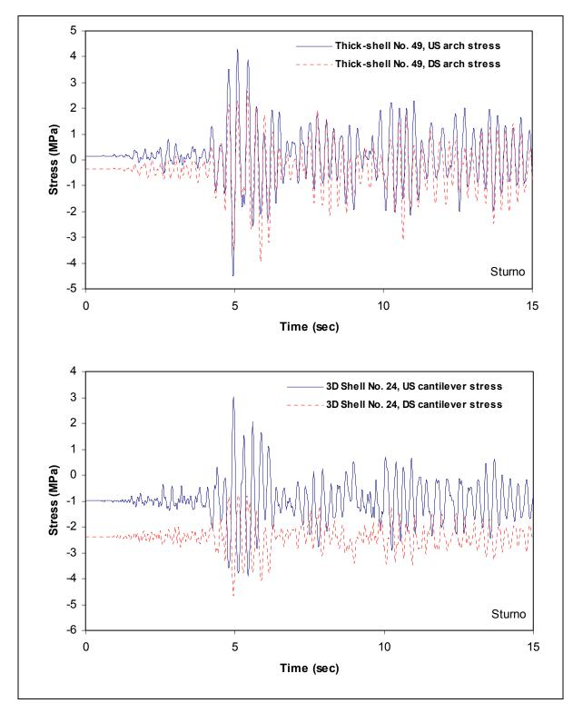
Figure 6.2-22. Time-histories of maximum arch and cantilever stresses and corresponding stresses on opposite face of the dam due to Sturno record plus static loads
