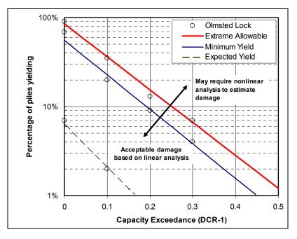
Figure 4-25. Acceptable percentage of pile yielding as a function of demand-capacity ratio levels in linear time-history analysis
