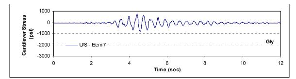
Figure 4-21. Time-history of maximum cantilever stresses for Dam-2
