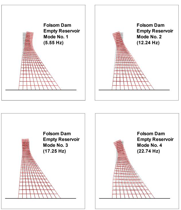
Figure 6.1-4. Mode shapes (empty reservoir)
