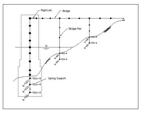
Figure 2-7. Finite element idealization of free-standing tower and access bridge
