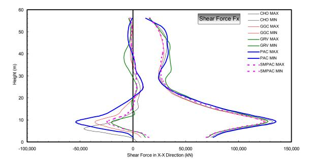
Figure 6.4-29. F<sub>x</sub> shear force diagram (normal to abutment)
