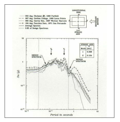
Figure 4-39. Horizontal design spectrum and the four scaled natural timehistories of the secondary set with 5 percent damping
