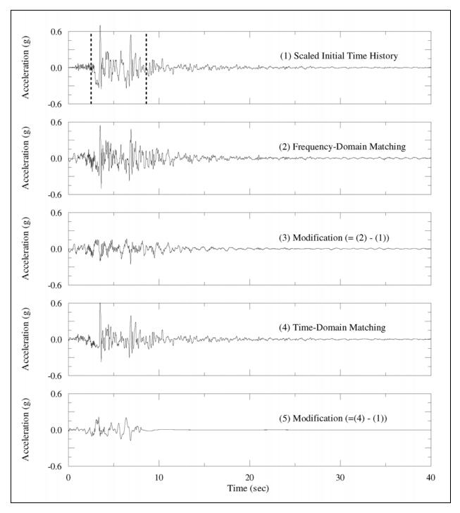
Figure C-8. Comparison of time-histories for SCSE recording (component 018E), 1994 Northridge earthquake (Sheet 1 of 3)
