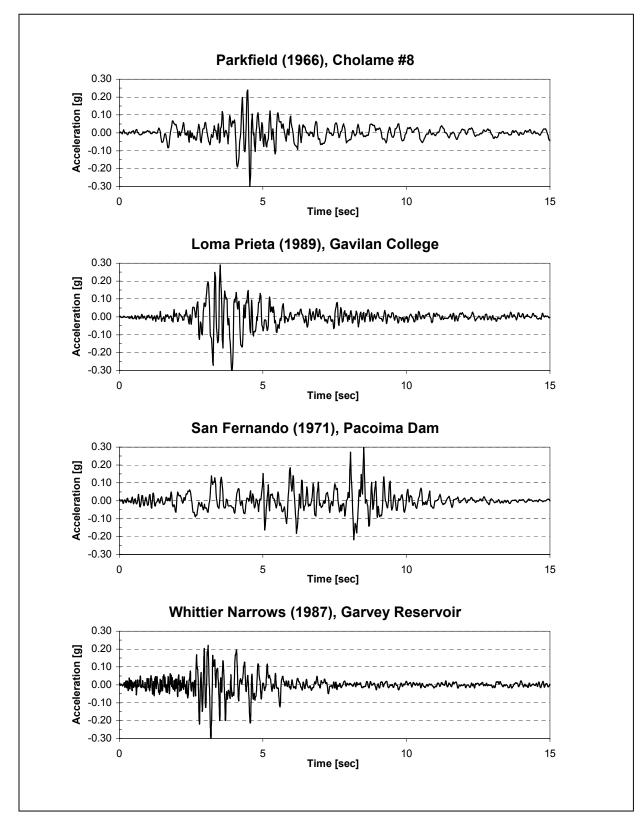
Figure 6.1-1. Ground motion acceleration time-histories used for analysis
