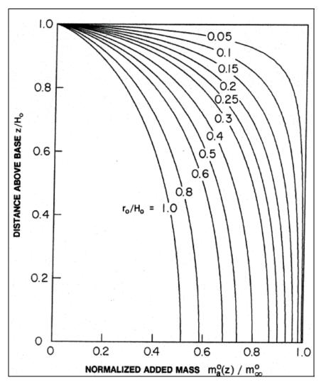
Figure 2-20. Normalized added hydrodynamic mass for circular cylindrical towers associated with surrounding water where z = distance above the base of the tower or pier,  $H_0$  = depth of the surrounding water,  $r_0$  = radius of the outside surface of the tower,  $m_{\infty}^o = \rho_w \pi r_o^2$  = the added mass per unit height of an infinitely long uniform tower of the same radius, and  $m_a^0(z)$  = the added mass for circular tower or pier surrounded by water (from Goyal and Chopra 1989)
