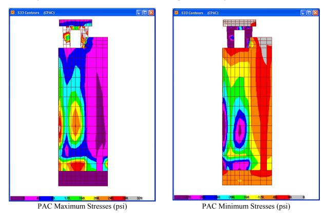
Figure 6.4-26. Vertical stresses in front face (upstream ) of tower for PAC
