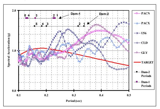
Figure 4-8. Horizontal and vertical smooth response spectra
