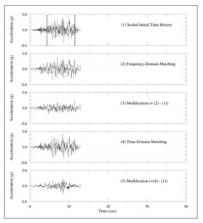
Figure C-5. Comparison of time-histories for Gazli recording (component 090E), 1976 Gazli earthquake (Sheet 1 of 3)
