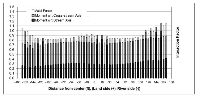
Figure 4-29. Combined static and dynamic interaction factors for H-piles under lower mitergate monolith subjected to MDE; expected yield case, FS = 1.0; distance to downstream face = 17 m (56.74 ft)
