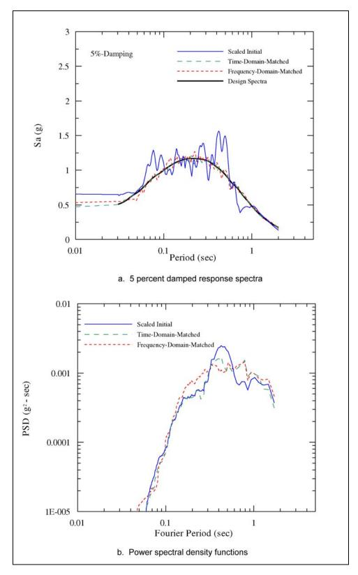
Figure C-19. Comparisons of response spectra and power spectral density functions for the scaled Pacoima Dam recording (component 254E), 1971 San Fernando earthquake, and the spectrum-compatible acceleration time-histories
