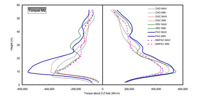
Figure 6.4-34. M<sub>z</sub> torque moment diagram
