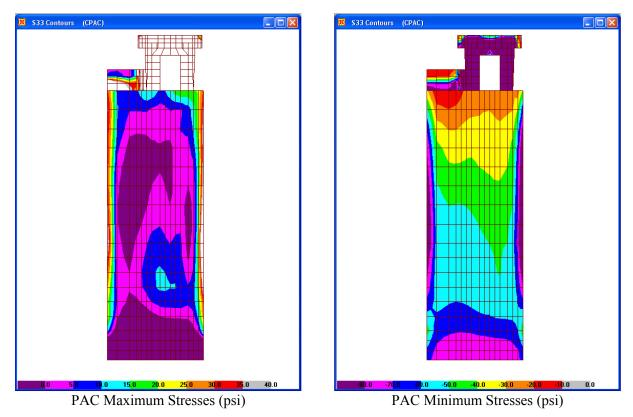
Figure 6.4-22. Vertical stresses in back face (downstream) of tower for PAC
