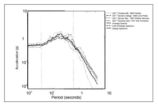
Figure 6.4-3. Target and scaled spectra, x-direction
