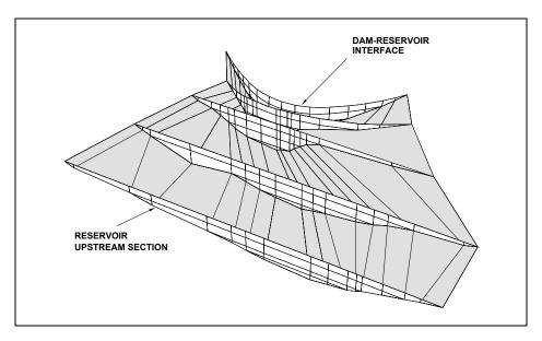
Figure 2-6. Finite element mesh for incompressible water developed to match reservoir bottom topography (shaded region)
