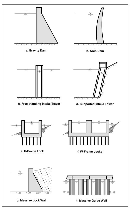
Figure 2-1. Types of concrete hydraulic structures
