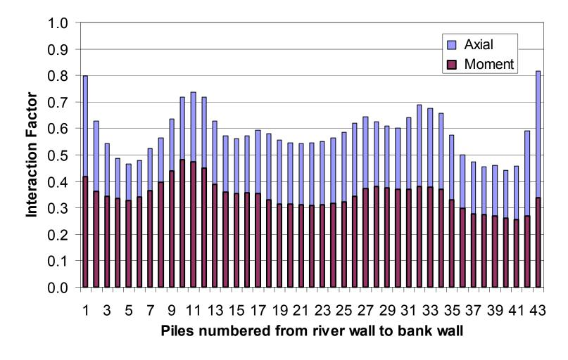
Figure 6.3-16. Envelopes of Maximum piles interaction factors for all load combination cases
