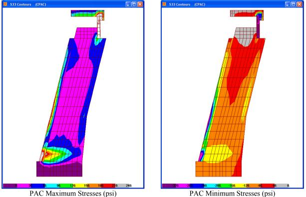
Figure 6.4-28. Vertical stresses in left face of tower for PAC
