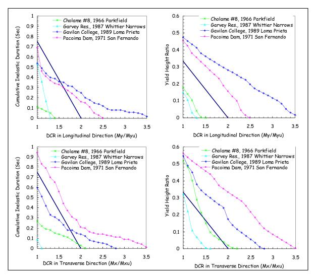
Figure 4-55. Structural performance assessment curves with 10 percent damping
