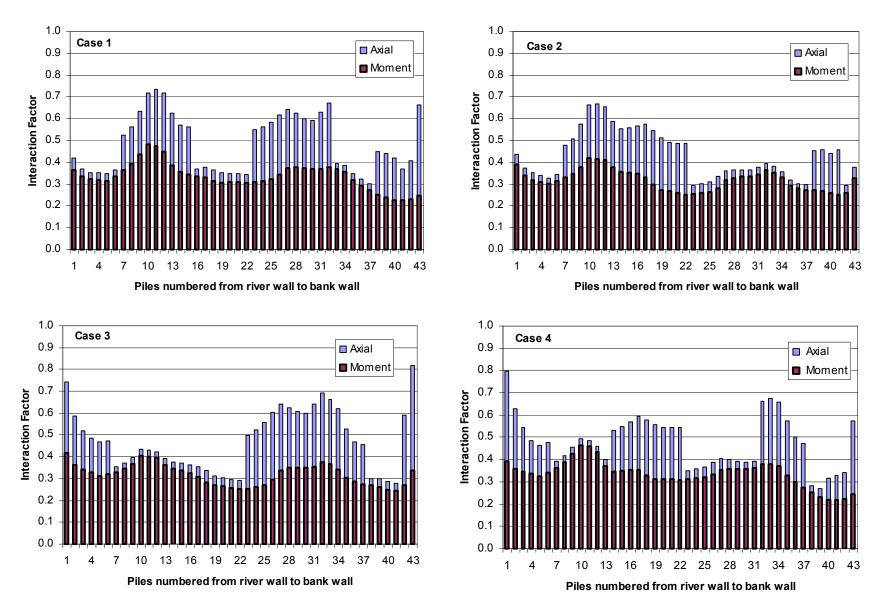
Figure 6.3-15. Maximum piles interaction factors for each load combination case listed in Table 6.3-4.
