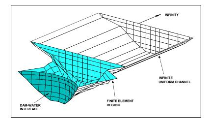
Figure 2-25. Finite element model of compressible water with absorptive boundary for Dongjiang Arch Dam, China (from Ghanaat et al. 1993)
