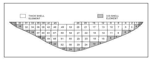
Figure 2-4. Finite element mesh of arch dam showing elements used in the dam
