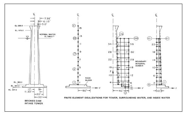
Figure 2-9. Finite element idealization of Briones Dam intake tower (from Goyal and Chopra 1989)
