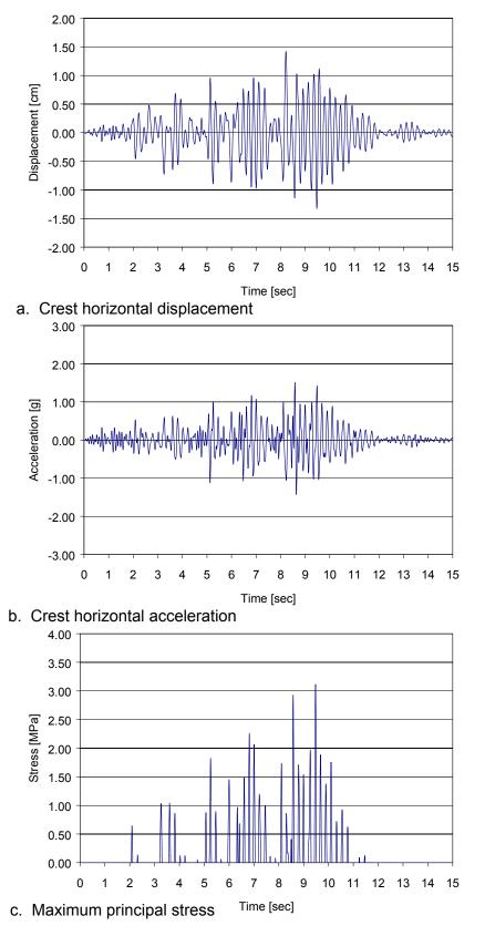
Figure 6.1-10. Relative displacement and absolute acceleration time-histories at the crest and maximum principal stress history at point B (San Fernando ground motion)
