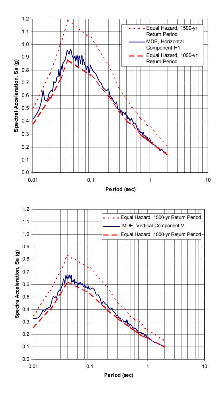
Figure 6.3-7. Comparison of 5%-damped rock motion response spectra with equal-hazard spectra
