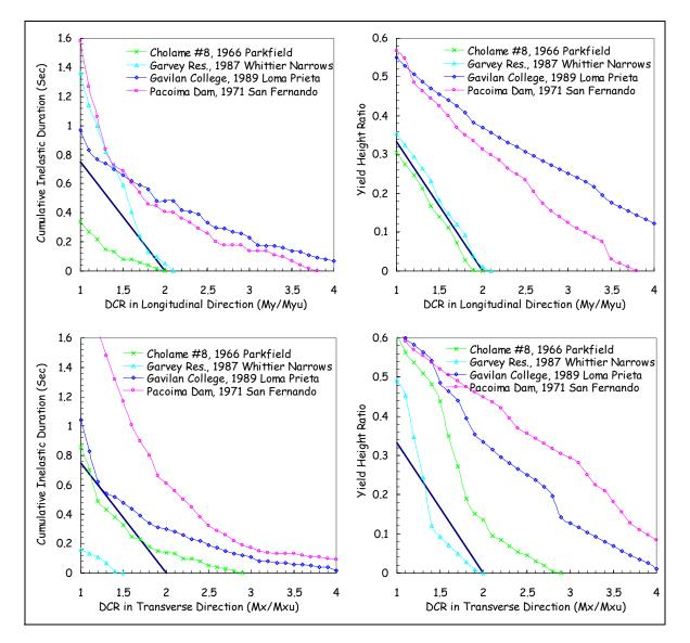
Figure 4-54. Structural performance assessment curves with 5 percent damping
