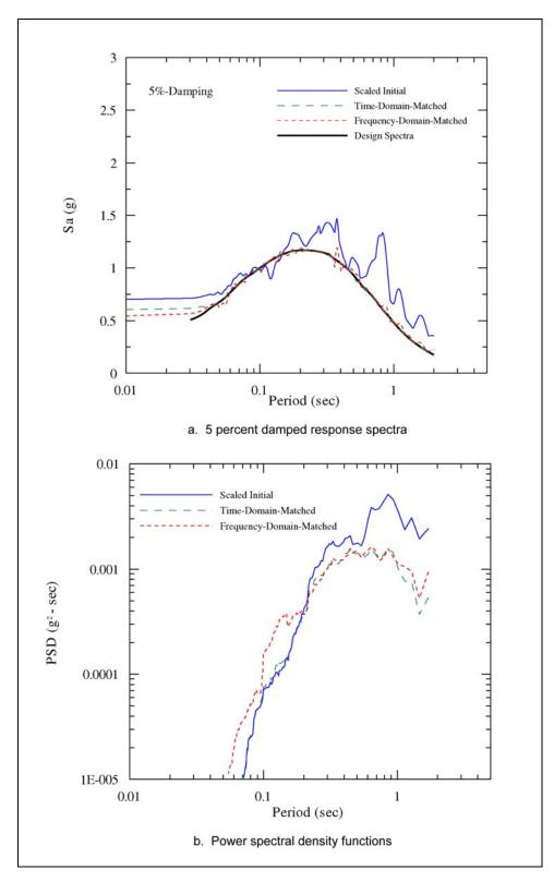
Figure C-18. Comparisons of response spectra and power spectral density functions for the scaled SCEC recording (component 018E), 1994 Northridge earthquake, and the spectrum-compatible acceleration time-histories
